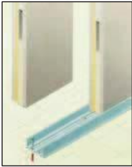
Assembly of cold rooms without floor
